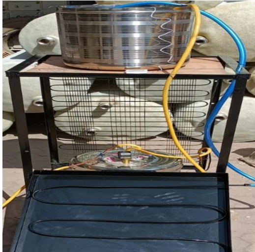
Figure 4. Developed adsorption refrigeration system.
