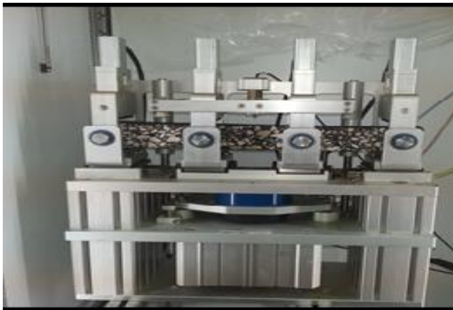
Figure 4. Four points bending beam test
