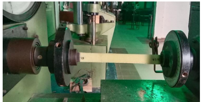
Figure 2. GFRP composite in torsion testing machine
