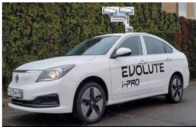
Figure10. An electric vehicle with a natural lighting system that uses sunlight, passing through optical fiber, installed on its roof
