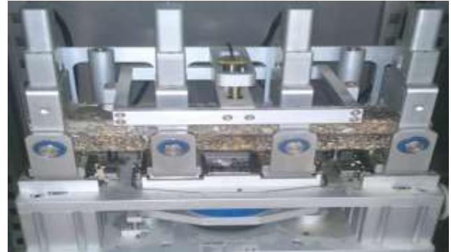
Figure 2. The four-point dynamic flexural bending beam test setup
