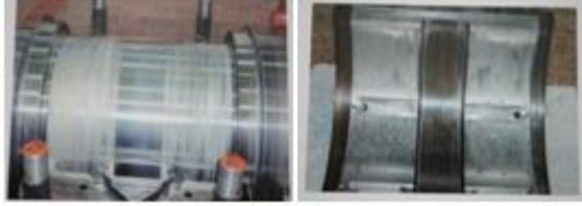
Figure 13. Pitting on the shaft and bearing of a short circuit alternator.
