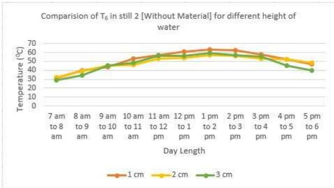
Figure 7. Variation of temperature in stills (Without material) for 1cm, 2cm and 3cm height of Water
