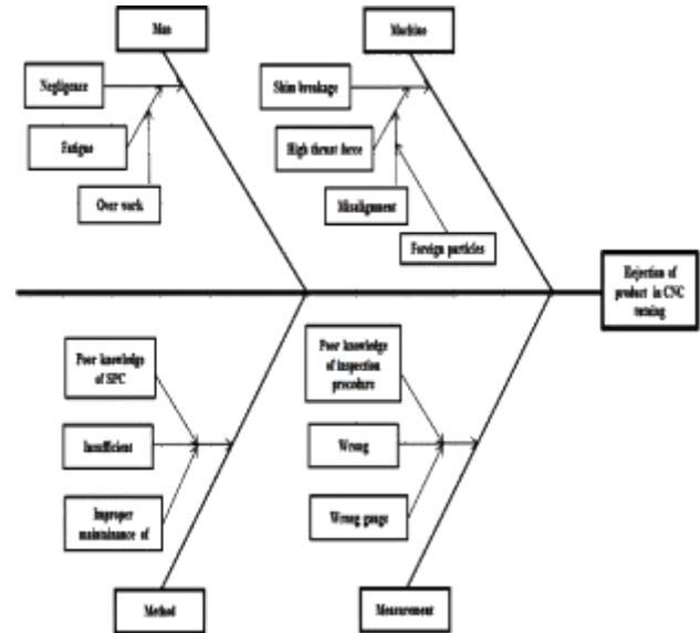
**Figure 5.** Cause and effect diagram for rejection of product in CNC turning
