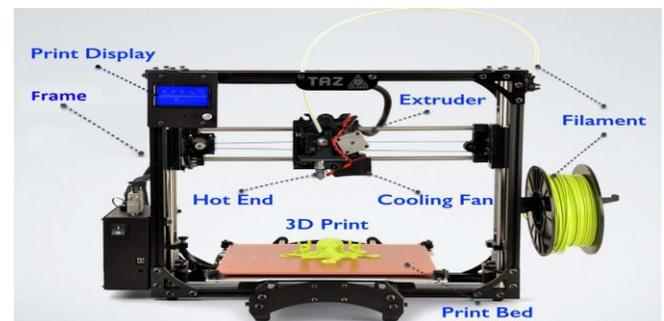
Figure 2. Main components used in FDM 3D printers [5]
