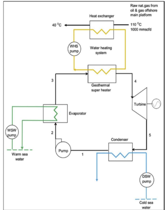
**Figure 1.** Schematic diagram of GeoTec Power Cycle [38]
